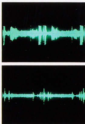
The results of oscilloscope tests for camera noise. Above is the wave pattern created by another camera. The extremely flat wave pattern of the Contax 137 MD Quartz shown below indicates the high degree of quietness.
