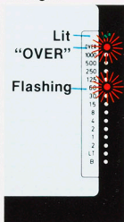
(*) mark flashes after proper exposure. When "OVER" flashes, smaller aperture must be used.
