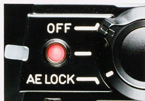
The Main Switch, showing OFF, ON (LED) and AE Lock positions.
