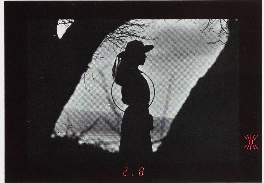
■ **When the LED indicating “B” flashes,** it will result in under-exposure. Since your subject is too dark, turn the aperture ring to a wider lens opening until the “B” lights steadily or a faster shutter speed is indicated before shooting. If the LED indicating “B” is still flashing even after the aperture is opened fully, switch to flash photography.
