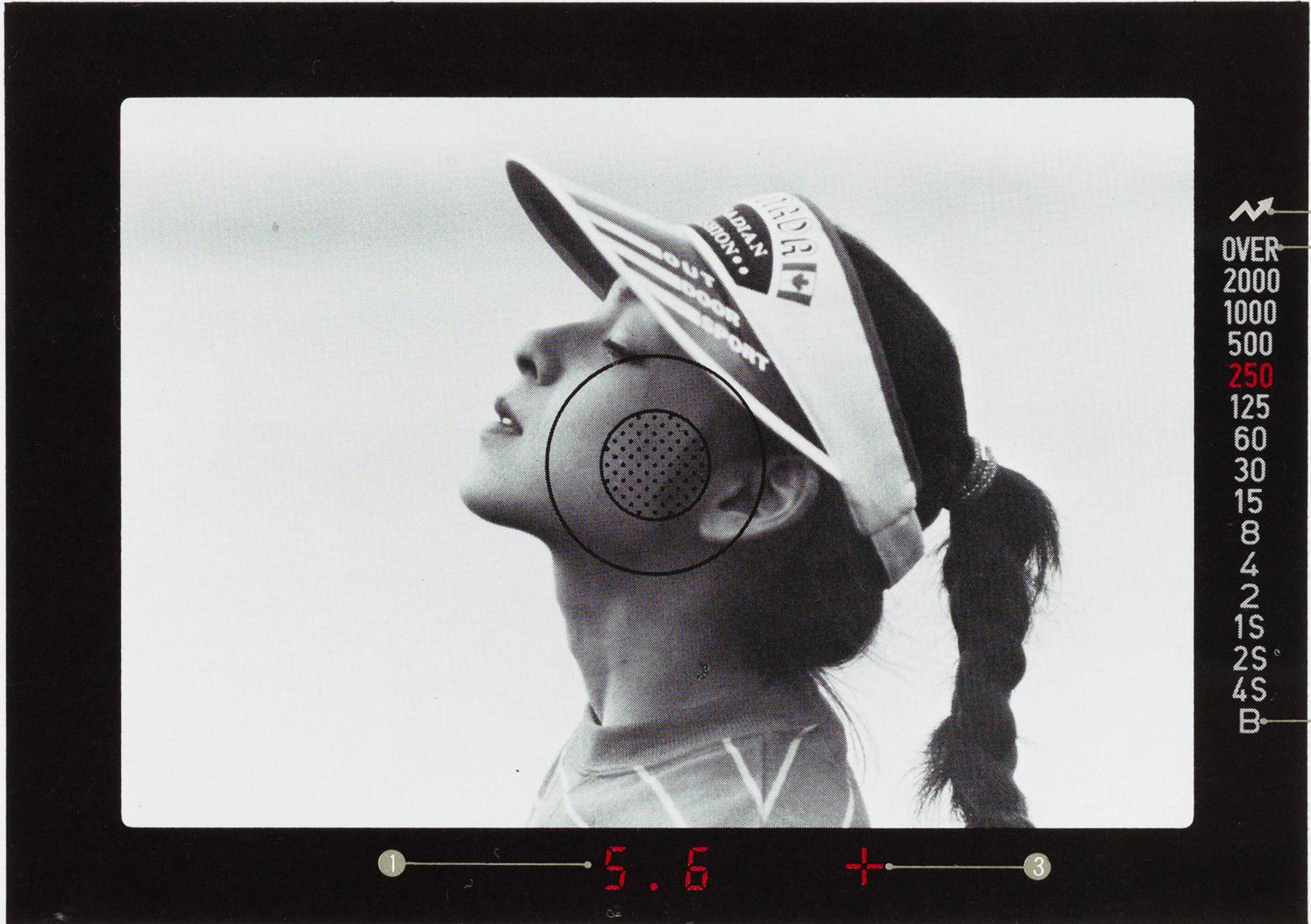
*The exposure data is given by means of an LED display system. The display is turned on by pressing the exposure check button, staying on continuously for 16 seconds. The LED display features a two-stage brightness control which automatically adjusts to the prevailing lighting condition, intensifying when bright and dimming when dark.*
