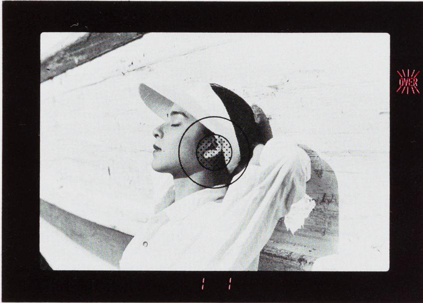
■ **When the LED indicating “OVER” flashes,** the picture will be over-exposed. Since the subject is too bright, turn the aperture ring until “2000” or a smaller number is indicated before shooting. If you stop down all the way and “OVER” is still indicated, it is necessary to use a neutral density filter, which is available as optional accessory.
