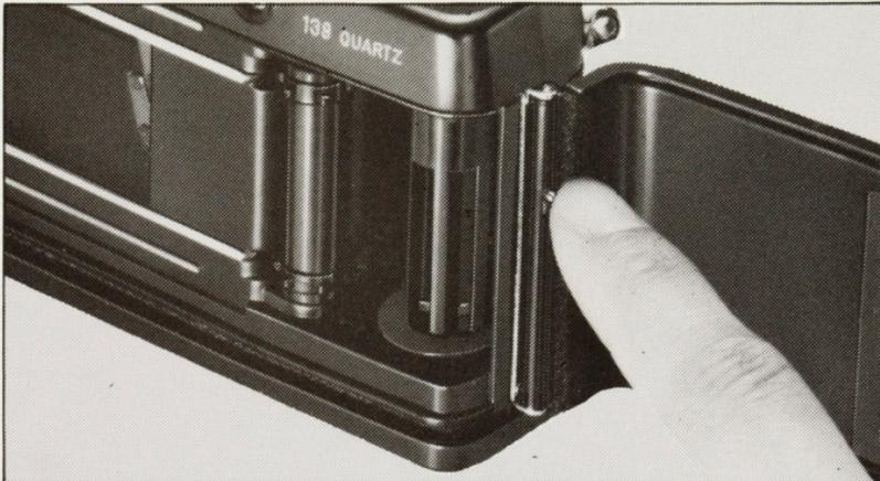
2 Insert the lower stud of the Data Back into the pivot socket near the camera base and notch the upper stud with the upper pivot socket while pressing down on the release lug of the Data Back.
