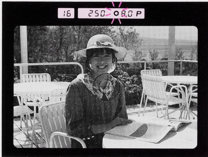
If the spot metering mode, you can take correctly exposed pictures with the AE Lock even if the subject is not located in the center of the picture frame.
