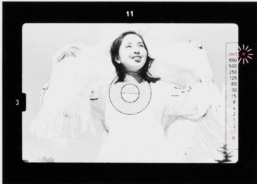
■ When the LED in the “OVER” position flashes, the picture will be over-exposed. Since the subject is too bright, turn the aperture ring until “1000” or a smaller number is indicated before shooting. If you stop down all the way and “OVER” is still indicated, it is necessary to use a neutral density filter, which must be purchased separately.
