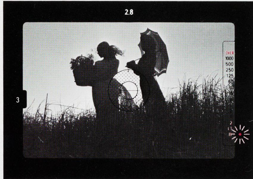
■ When the LED in the “B” position flashes, the subject is too dark, turn the aperture ring in the direction of smaller numbers (larger openings) until “LT” or a faster shutter speed is indicated before shooting.
