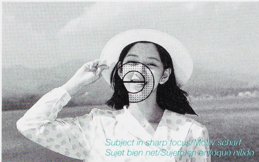
*This camera is normally equipped with a focusing screen FW-1 (horizontal split-image/microprism type). Focusing can be done on a horizontal split-image spot in the center, on the microprism collar around it, and on the surrounding matte area.*
